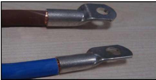
Figure 4: A type of lug that was directly connected to the cable end and that was correctly assembled.
