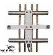
The LMC intelligent wire rope sensor precisely monitors the load in traction elevators. Perfect for modernizations, it mounts on the hoist ropes in as little as five minutes. Calibration is automatic - no test weights are required. It is accurate to within 0.5% of total weight.
