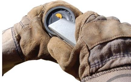
(4) Once the nipples are removed, the lubricators can be screwed into the fitting. Snugly hand-tighten the lubricators.
